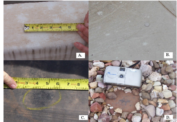
Figure 9. A) Location 35-Large hail impact on PVC-covered parapet with no apparent damage; B) Location 88-Hail impact marks visible on TPO membrane surface, but no fractures visible; C) Location 27-Insulation dented, but no fracture in EPDM membrane at 2.0 inch diameter impact; D) Location 31-No fracture visible in EPDM membrane where stone ballast had been displaced by large hailstone impact.
