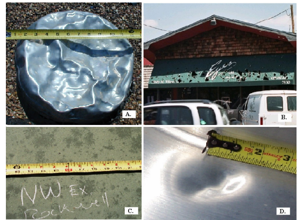
Figure 1. A) Buckled vent cap; B) Awning punctured by hailstones; C) Hail impact spatter marks; D) Large dent in vent hood.
