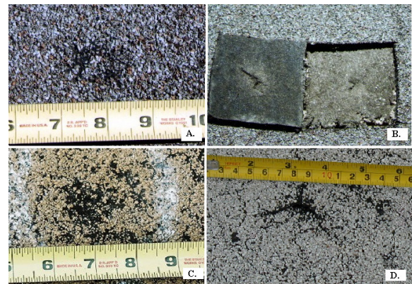
Figure 6. A) Location 26-Impact-caused bruise observed on surface of SBS membrane; B) Location 26-Fracture in underside of membrane at Photo A; C) Location 76-Impact-caused bruise with recent granule loss on surface of SBS membrane; D) Location 95-Impact-caused fracture observed on surface in blistered location.
