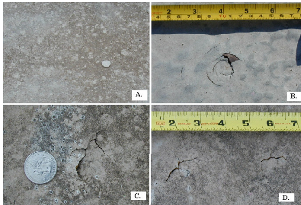
Figure 7. A) Location 100-Hailstone impacts had removed surface grime, but not fractured SPF coating; B) Location 94-Impact-caused concentric circular fractures; C) Location 97-Hail impact spatter mark at starburst fracture on indentation in SPF; D) Location 97-Two adjacent hail-caused fractures in SPF coating.
