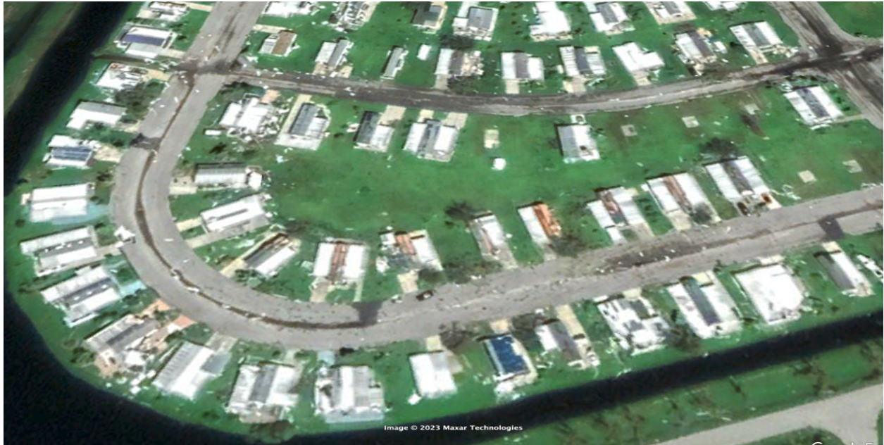
Figure 3: This photo shows the subdivision immediately east of that shown in Figure 2. There was more damage here to units that were built between 1998 and 2004. Other sections were completed after 2004.
