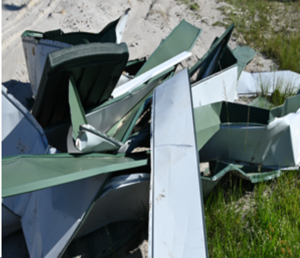
Photo 89: The debris pile shows lack of fasteners
