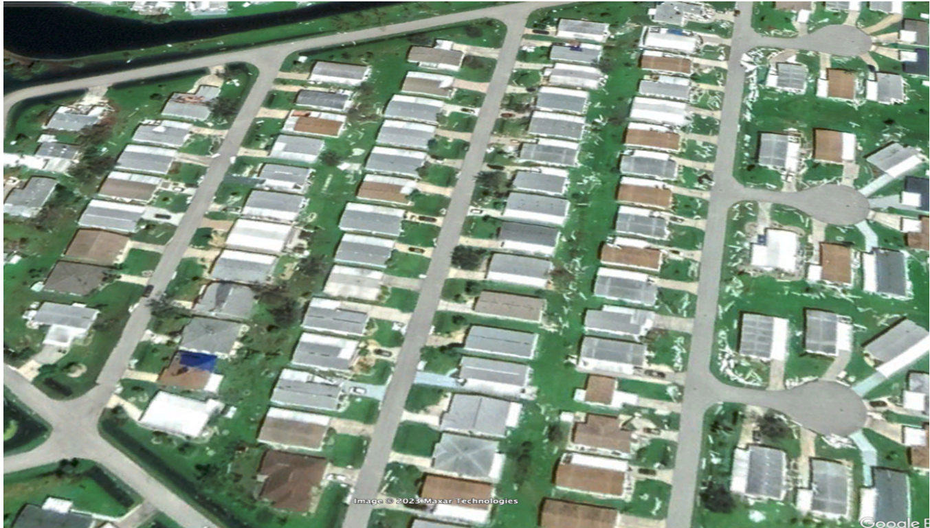
Figure 2: This is the area immediately east of that shown in Figure 1. It shows some debris but little or no roof damage. This section was developed from 2004 to 2016 with units around the cul-de-sacs built last.
