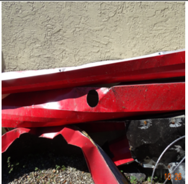
Photo 165: Approximately 18" O.C. Fastening
